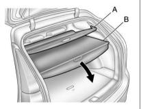
The shade can be set in two positions. It can be set in a half way open (A) position for loading objects into the rear compartment, or the lower (B) position to conceal objects in the rear compartment.
